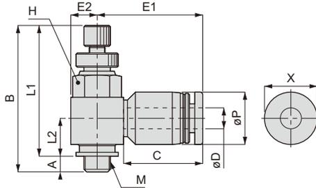
Appearance dimension for taper pipe thread (R)
