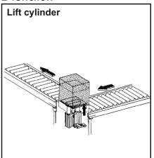
Special design which stands the large one-sided load. Lifts the work carrier at a fixed point not changing the posture.
