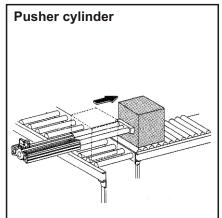
Long strokes available, the highly precise pushing work transfers and places a work carrier and changes the direction.
