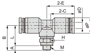
Appearance dimension for taper pipe thread (R)
