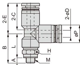
Appearance dimension for taper pipe thread (R)
