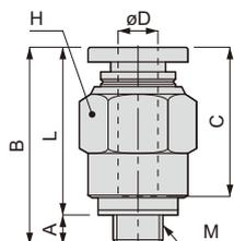
Appearance dimension for taper pipe thread (R)
