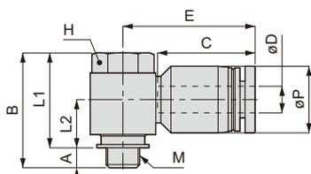
Appearance dimension for taper pipe thread (R)
