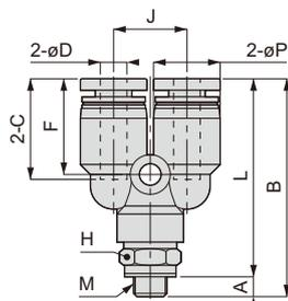
Appearance dimension for taper pipe thread (R)
