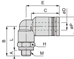
Appearance dimension for taper pipe thread (R)
