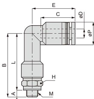
Appearance dimension for taper pipe thread (R)
